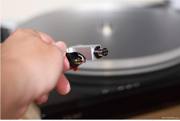
Install the cartridge cover, which is already locked on the cartridge when shipped from the factory.
