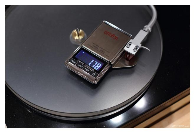
Re-adjust the MC cartridge after replacing it.
