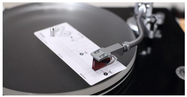
Adjust the needle pressure. The standard of Ortofon 2M RED MM is 1.8 grams. It is ideal to set a close value first and then make adjustments after actual listening.
