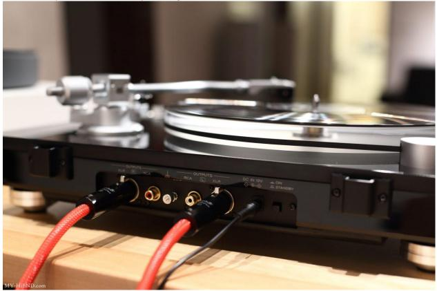
The space between the input and output of the PE-505 is quite large, so it is no problem to use fever wires with larger terminal diameters.
