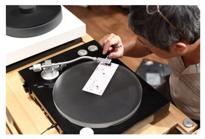
It provides XLR balanced output and corresponds to the MC phono cartridge. After completing the basic adjustment of the turntable, fine-tuning must be done through actual listening, so the next step is to unbox the matching phono stage TEAC PE-505. PE-505 is closely matched with TN-5BB in design. TN-5BB has XLR balanced output, while PE-505 has XLR balanced input and can be used with MC cartridges. If these two pieces of equipment are used together, all Basically no functionality is wasted.
