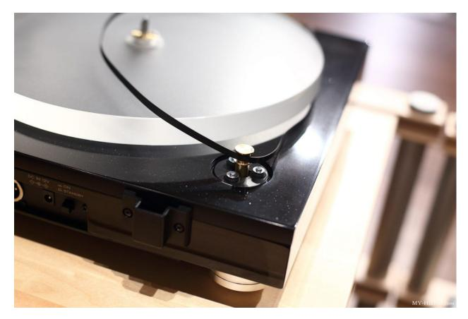
Automatic arm raising button. When the light is on, it means that the tone arm has not been lowered. When the tone arm is lowered, the light will go out. Above is the speed adjustment, with a total of 4 levels, static, 33.3, 45, and 78 rpm.
